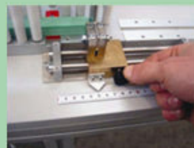
Adjustable stop to modify fabric first hole distance from edge.
