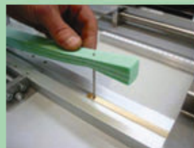
Scale and reference pin for calculating position and number of holes on fabric.
