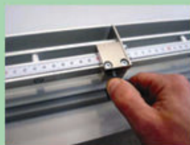
Adjustable stop to determine fabric cutting size.
