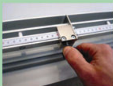
Adjustable stop to determine fabric cutting size.
