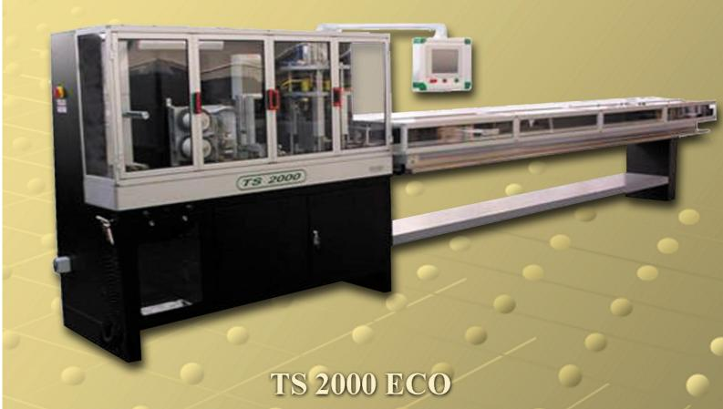
The NEW TS2000 ECO is a fully automatic machine for the production of vertical blinds equipped with a touch screen act ivated computer cutting, punching, folding and welding by ultrasonic with an automatic insertion of the hangers. The machine is able to process with a precision of 0,1 mm and a productivity of 240 louvers per hour (average size). Soft Trevira CS fabrics can be processed exactly like coated fabrics, since our machine is
